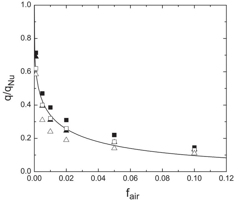
**Figure 7.4:** Reduction of the heat transfer from condensing steam by the presence of a certain fraction of air:  $f_{\text{air}} = \rho_{\text{air}}/(\rho_{\text{air}} + \rho_{\text{vapor}})$  [137]. Black and open symbols denote the data for temperatures of  $100^\circ\text{C}$  and  $82^\circ\text{C}$ , respectively. Squares represent data for  $T_{\text{sat}} - T_w = 5^\circ\text{C}$ , triangles those for  $T_{\text{sat}} - T_w = 15^\circ\text{C}$ .
