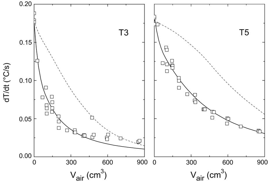
**Figure 7.6:** Temperature change per unit of time ( $dT/dt$ ) at the positions of T3 and T5 of the ETS (see figure 7.2) as a function of the volume of air injected just before the final inlet of steam. The derivatives  $dT/dt$  are calculated at the start of the sterilization phase. The open squares denote the experimental data, the dashed and solid curves reflect the corresponding model predictions assuming ideal and non-ideal film condensation, respectively.
