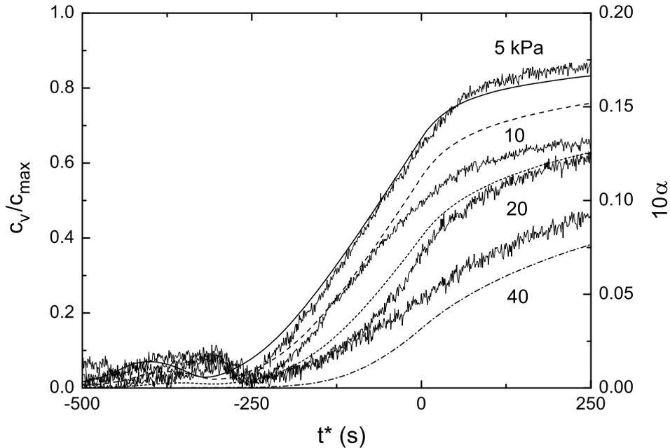
**Figure 6.6:** Moisture concentration at the closed end of the test tube as a function of time for generic processes with VCP's of 5, 10, 20, and 40 kPa, respectively. The corresponding results of the modified model are represented by the solid, dashed, dotted, and dashed-dotted black curves. The time for the individual processes has been shifted such that  $t^* = 0$  corresponds to the start of the sterilization phase.
