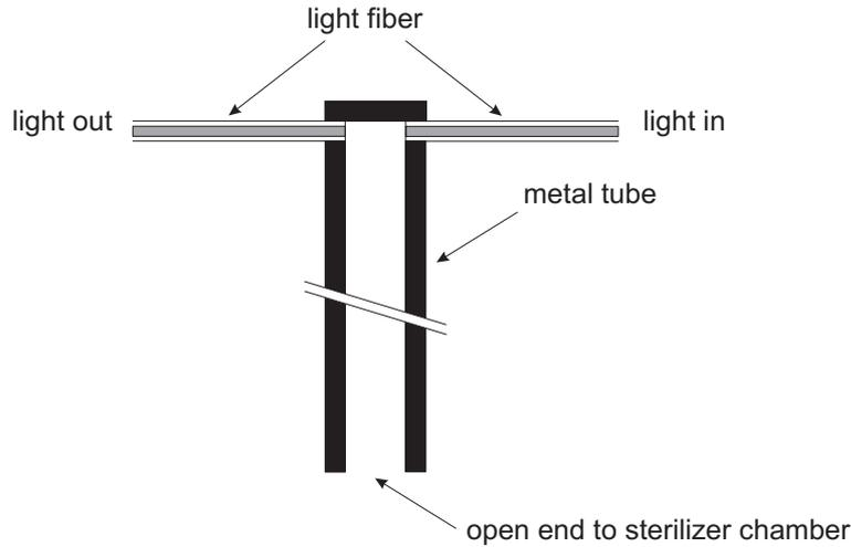
**Figure 6.4:** Schematic representation of the test tube with water vapor sensor. The tube has an open and a closed end. It is positioned with the closed end pointing upwards in the test sterilizer and the open end downwards. At the closed end of the tube ( $x = L$ ) an infrared light beam is emitted into the tube via a glass fiber. At the opposite side of the tube a second fiber is receiving the light that is transmitted through the gas mixture in the tube.
