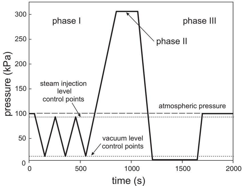
**Figure 6.1:** Schematic pressure curve of a surface steam sterilization process. Phase I: replacement of air by water vapor; Phase II: actual sterilization phase involving a predetermined combination of temperature and pressure during a certain time; Phase III: returning the steam sterilizer to a safe mode and drying of the load.
