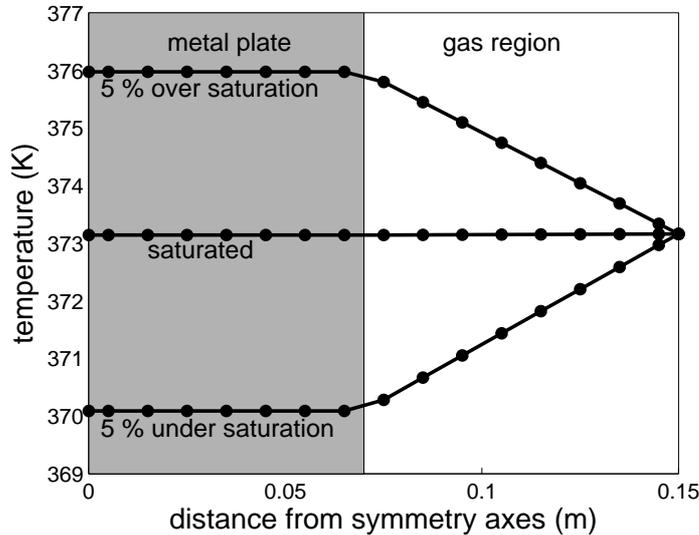
**Figure 8.3:** Steady state solution of the system presented in figure 8.2 with an initial temperature of 293.16 K and boundary conditions on the open boundaries at  $x = 0.15$  m given by  $T = 373.16$  K and a pressure of 202.07 kPa. On the inlet boundary ( $x = 0.15$  m) different gas mixes are imposed with over-, under- and saturated with water vapor as tabulated in table 8.1. The black dots in the curves represent the grid at which the temperature is calculated (figure 8.2).
