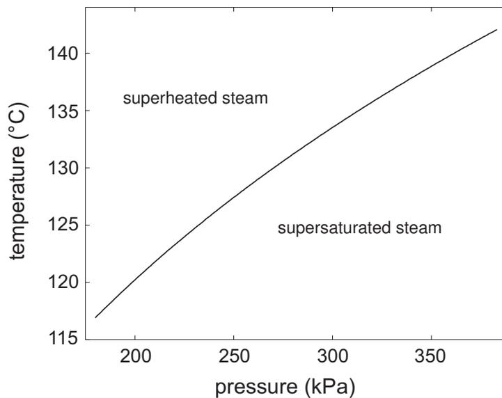
**Figure 4.1:** Theoretical temperature of 100 % saturated steam ( $T_p$ ) calculated from the pressure ( $p$ ) [72]. Above the curve the steam is superheated and below the curve the steam is supersaturated (often called wet steam).
