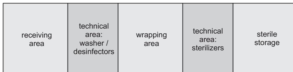
**Figure A.1:** Schematic layout of a CSSD. Medical devices to be processed arrive in the receiving area. After the first check and registration they are loaded in a washer-disinfector. At the wrapping side the washer-disinfector is unloaded and the instruments are wrapped. The wrapped instruments are loaded in the sterilizer. After the process the sterilizer is unloaded in the sterile storage.
