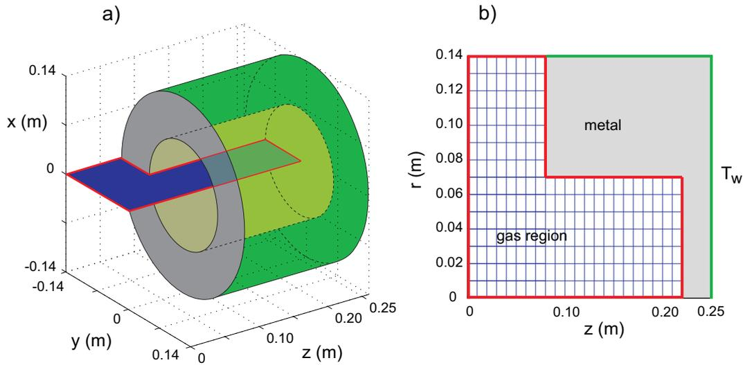
**Figure 8.4:** Geometry of the cylindrical metal bar with a channel that is open at one end. The blue rectangle represents the grid used for calculation and is given in more detail in figure b. The gas distribution is calculated within the red region.
