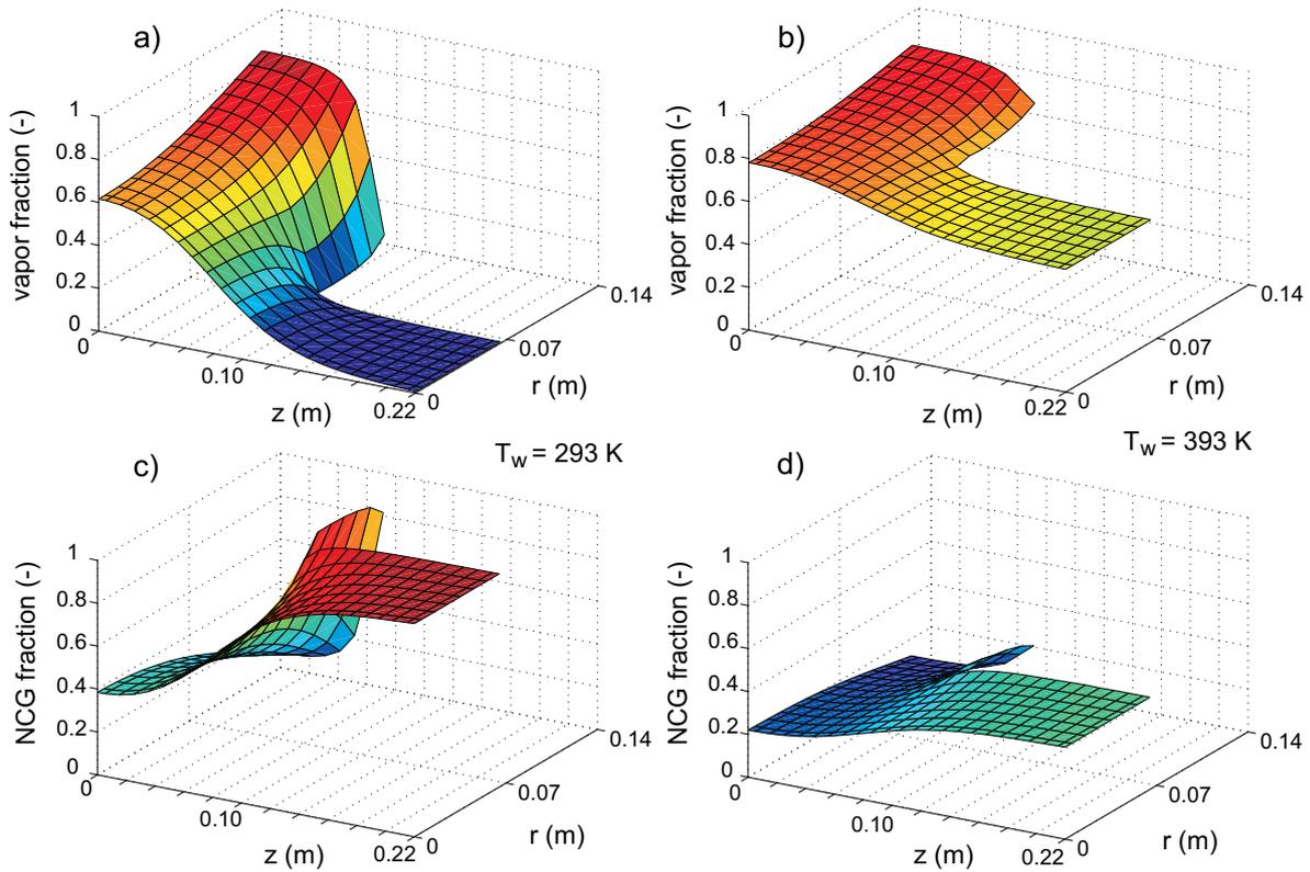
**Figure 8.5:** Gas distribution within the metal cylinder depicted in figure 8.4. For the calculations all conditions were kept the same except the temperature on the outside boundary of the metal cylinder ( $T_w$ ). In the figures a) and c) results are presented for  $T_w = 293$  K, in the figures b) and d) those for  $T_w = 393$  K.
