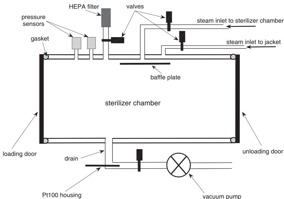
**Figure 2.1:** Schematic representation of a vacuum assisted steam sterilizer.
