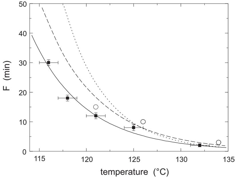
**Figure 5.5:** Various time-temperature combinations that might be used for steam sterilization processes. The black squares represent the data reported by Perkins [88], the open circles represent those given by the MRC [31]. The solid curve is a fit of equation 5.19 to the data of Perkins. The dashed curve reflects the effect of increasing the sterility by 50%, the dotted curve represents the effect of increasing the inactivation energy by 30%.
