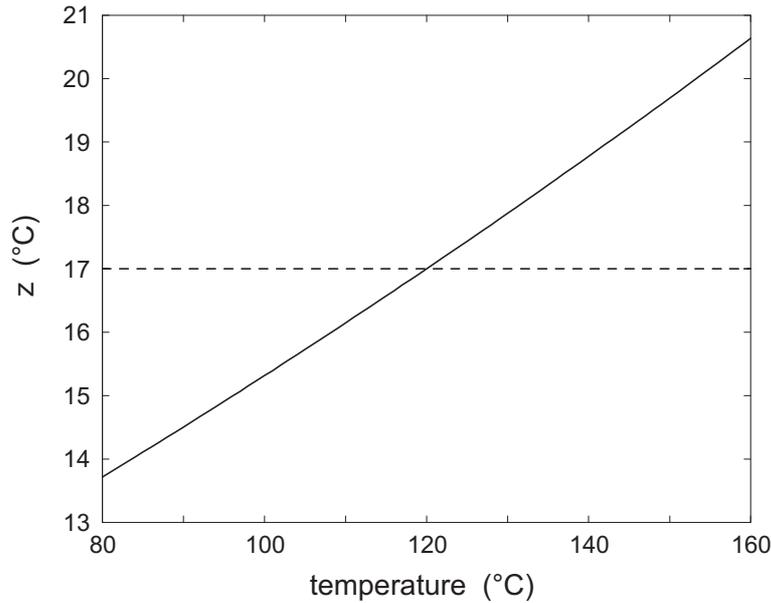
**Figure 5.2:** Variation of the resistance coefficient  $z$  with temperature. The horizontal dashed line represents the constant value  $z = 17^\circ\text{C}$  used in various theoretical models [18, 19, 59]. The solid curve represents  $z(T)$  calculated from equation 5.16, using  $T_{\text{ref}} = 120^\circ\text{C}$  and  $z_{\text{ref}} = 17^\circ\text{C}$ .
