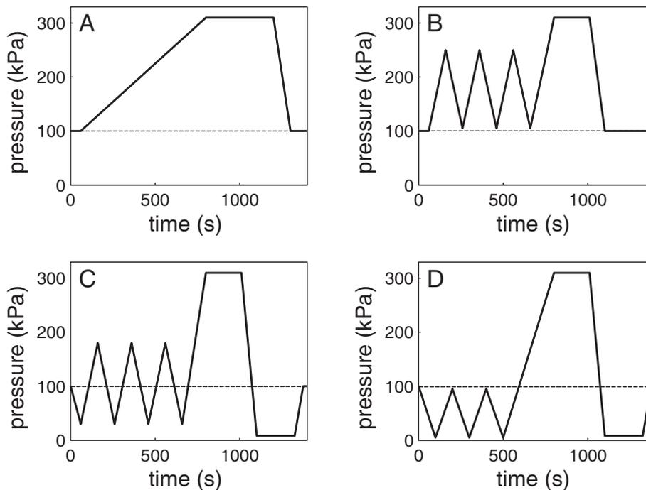
**Figure 2.3:** Schematic representation of various sterilization processes. The horizontal line at 100 kPa represents the atmospheric pressure. A) Flush process. B) Super-atmospheric pulsing. C) Trans-atmospheric pulsing. D) Sub-atmospheric pulsing [52].
