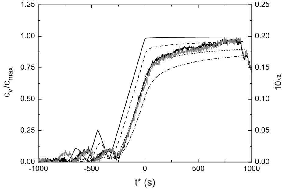
**Figure 6.5:** Experimental data for a process with 3 VCP's of 5 kPa (black) and a process with 4 VCP's of 10 kPa (grey). The solid black curve denotes the model prediction for the first process. The predictions of the adapted model are denoted by the dashed, dotted, and dashed-dotted curve for  $\tau = 30$ , 60, and 90  $\text{s m}^{-1}$ , respectively.
