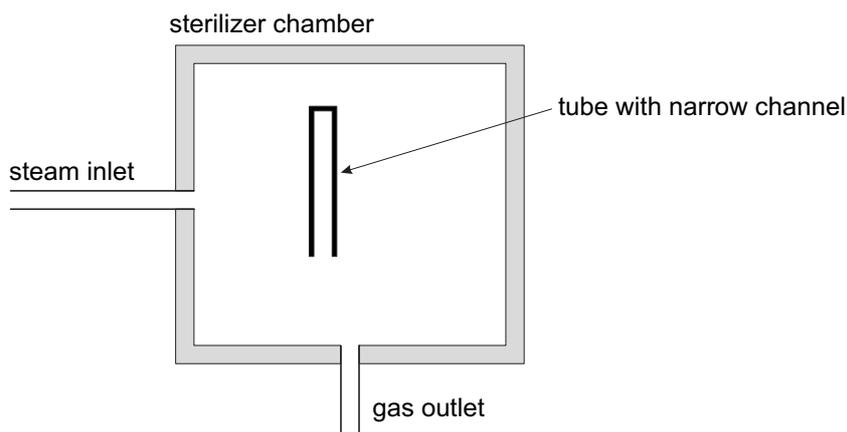
**Figure 6.2:** Schematic representation of the model used in the computations. During pressurization steam is injected and the outlet is closed (see figure 2.1). During evacuation the inlet is closed, the vacuum pump is switched on and the outlet is opened. A tube with a narrow channel is positioned in the steam sterilizer chamber, the closed end up and the open end down. The tube has no direct thermal contact with the wall.
