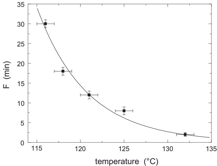
**Figure 5.3:** Time-temperature combinations to achieve sterility for aqueous liquids given by Perkins [88] (black squares) and a fit of equation 5.19 to these data. The initial number of organisms  $N_0$  is taken equal to  $10^6$ .
