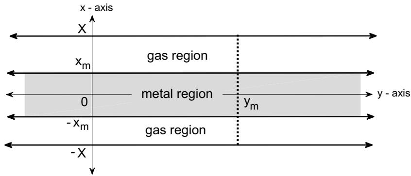
**Figure 8.1:** A metal plate in a gas region. The  $z$ -axis is oriented perpendicular to the surface. Both the  $y$ - and  $z$ -axis extend into infinity and are symmetry axes. The metal region extends from  $0 \leq x \leq x_m$  and the gas region from  $x_m < x \leq X$ . The origin  $(0,0,0)$  is the symmetry point.
