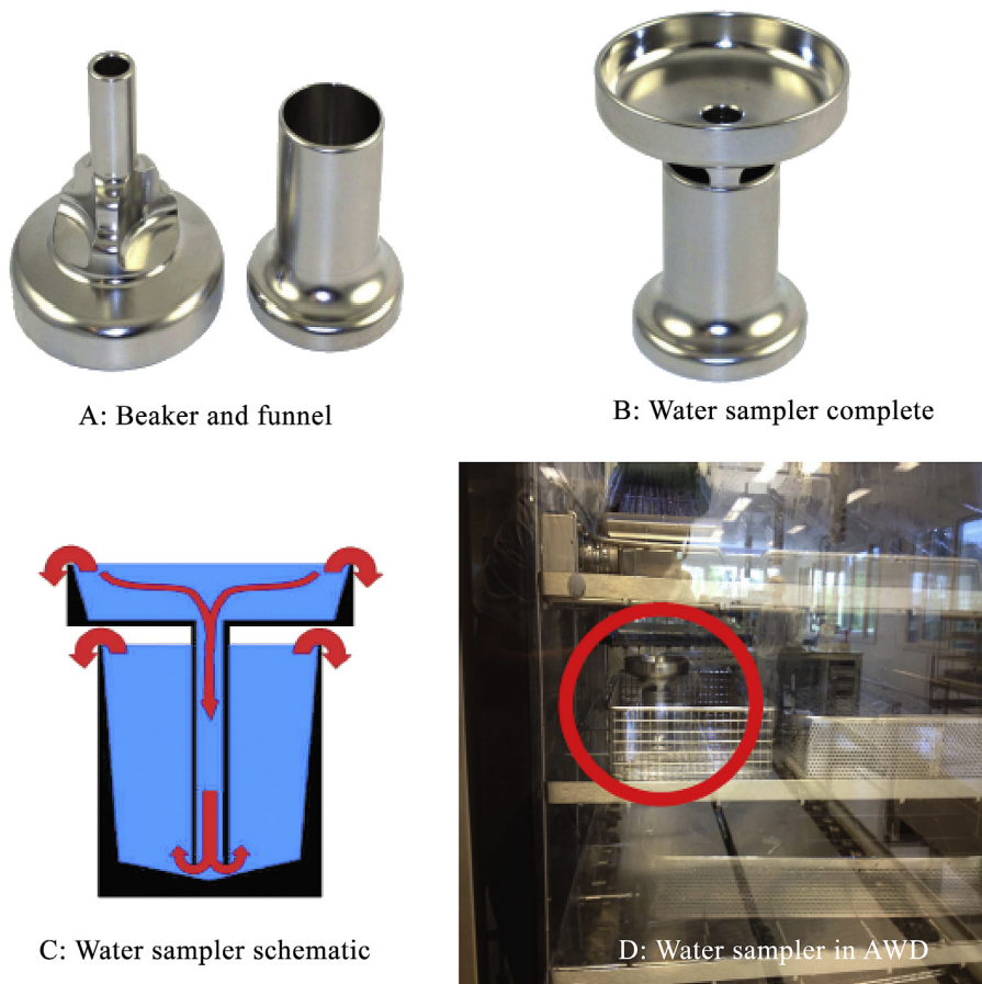
Figure 1. Water sampler (WS). (A) Components of the WS: a funnel and a beaker. The funnel is so wide that water can only access the beaker via the funnel. (B) WS as used in an automated washer-disinfector (AWD). The stainless steel WS is constructed such that it does not tip over during an AWD process, e.g. by the force of a water spray. (C) The principle of the WS: the red arrows indicate the water flow direction. During a process, water will be collected by the funnel and flow into the beaker. The funnel outlet extends almost to the bottom of the beaker. The bottom of the rinse water collector is constructed such that the water present in the beaker is pushed upwards and out of the beaker. Hence, at the end of a process the WS essentially contains the last rinsing water. (D) The position of the WS in all AWD tests in this study.
